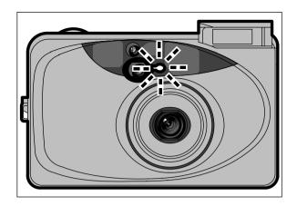
The self-timer lamp will begin to blink approximately seven seconds after being illuminated, and the shutter will be released approximately three seconds after that.
